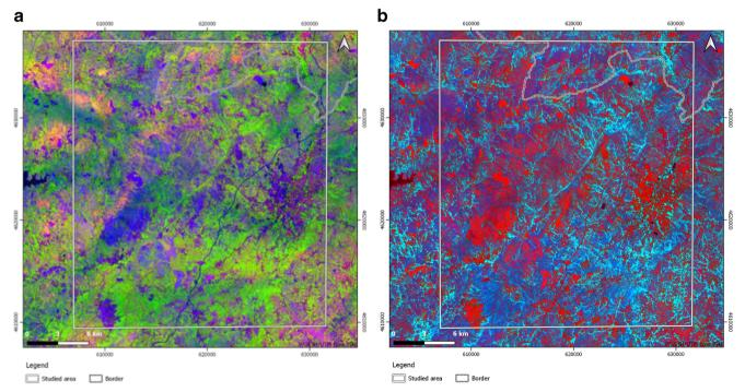
Fig. 5 RGB composite images using band ratios to discriminate hydrothermally altered areas. a Sabin's ratio (RGB 4/2, 6/7, 6/5). b Kaufmann ratio (RGB 7/5, 5/4, 6/7)
