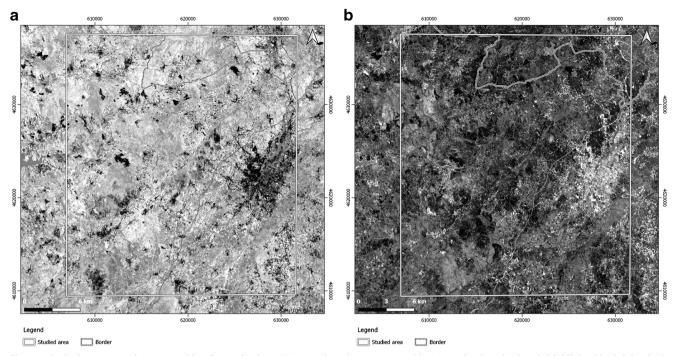
Fig. 7 Principal component images resulting from selective PCA. a Hydroxyl (H). b Iron oxide (F). Each mineral subset is highlighted by bright pixels
