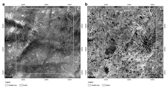
Fig. 4 Highlighted altered minerals through band rationing. a 4/2 ratio image mapping iron oxides in bright pixels. b 6/7 ratio image mapping hydroxylbearing minerals in bright pixels
