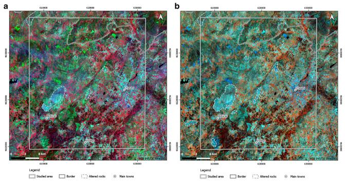
Fig. 3 False color composites enhancing the different spectral signatures in the study area. **a** RGB 573—vegetation is shown in shades of red, urban areas and ploughed fields in light blue to light green, and rock outcrops in shades of green to light blue. The intense light blue color observed in rock outcrops is interpreted as alteration, highlighted with
