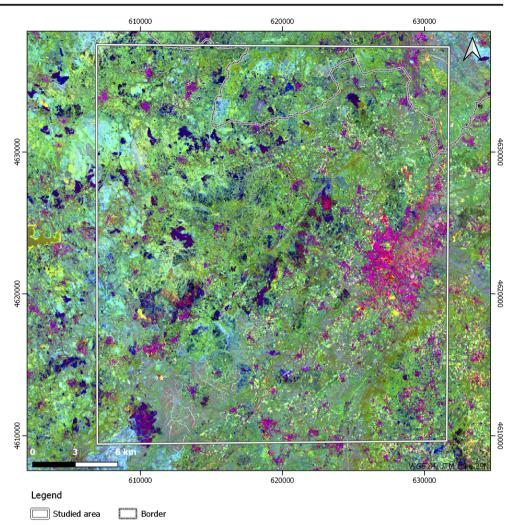
PC4 image is negated to highlight hydroxyl-bearing minerals in bright pixels, and it was used as a hydroxyl image (H) (Fig. 7a) in the final RGB combination. This image has a negative contribution from vegetation in the NIR band (band 5), which has a similar response to hydroxyls in the SWIR bands.
