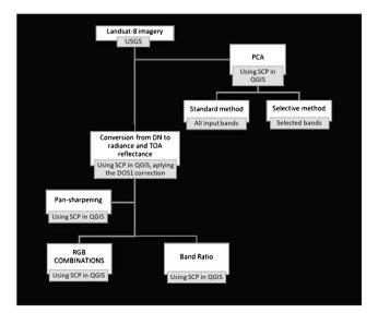
Fig. 2 Schematic diagram of overall workflow
